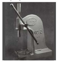
Greenerd has been designing and building arbor presses for over 100 years. Available in 46 hand-operated lever, ratchet, and pilot wheel models, they are ideal for assembling, staking, punching, bending, broaching, testing, forming, straightening, blanking, and compressing. The most accurate arbor presses made, they are designed with rugged cast-iron construction to handle even the toughest, heavy-duty jobs.
